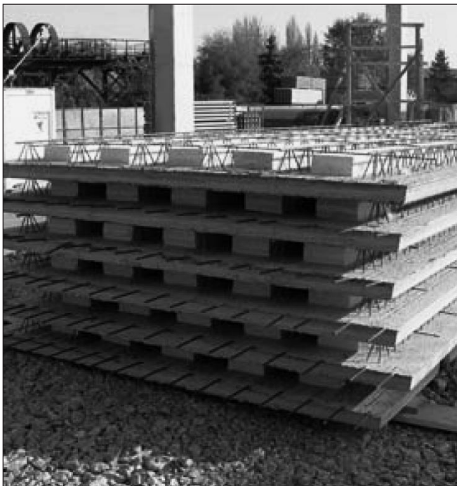
Fig. 7: Styropor Lightened Floor Planks with Truss
